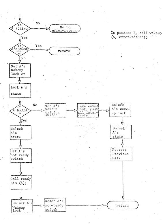
Figure 2. Complete Flow Diagram for Wakeup
