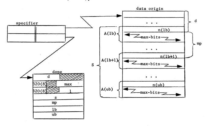
The dope specifies a 1-dimensional array which looks (except for the id code) like an array of unpacked, non-varying strings of length max. The current length of the string A(i) is stored just preceding the string, n(i) in the diagram. Each length may be different, however, each must be  $\leq \max$ .
