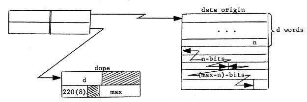
where  $\underline{d}$  is the offset (in words), 220(8) the id code,  $\underline{max}$  the maximum length of the string (in bits), and  $\underline{n}$  the current length (in bits). A number of memory locations sufficient to contain a string of maximum length is initially allocated  $\underline{d}$  words from the data origin. The string always begins at bit 0 in the word at data\_origin+d. The word immediately preceding this (data\_origin+d-1) contains the current length of the string.
