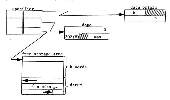
A long varying string datum is always unpacked and is located in a free storage area, while auxiliary data, which specifies the position of the string in the free area, is found at the data origin. The addressing offset in the dope is always zero.
