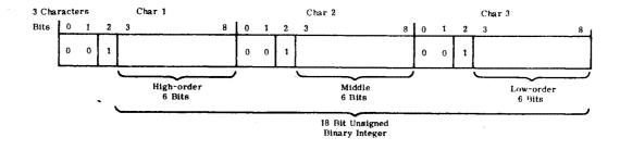
Unique ID (UID) format is used to transmit 18-bit node numbers.
