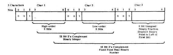
Scaled Fixed Point (SCL) format is used for numbers with fractional parts. It has the same range as the DPI format, but is accurate to fractional parts of 1/64.
