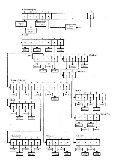
Figure 2 A Typical Graphic Structure Organization
